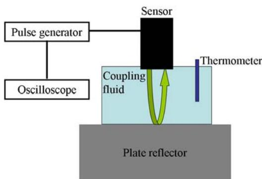
Fig.2 The experimental setup.
