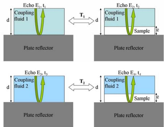
Fig.1 The method uses two coupling fluids and breaks out into four echoes.
