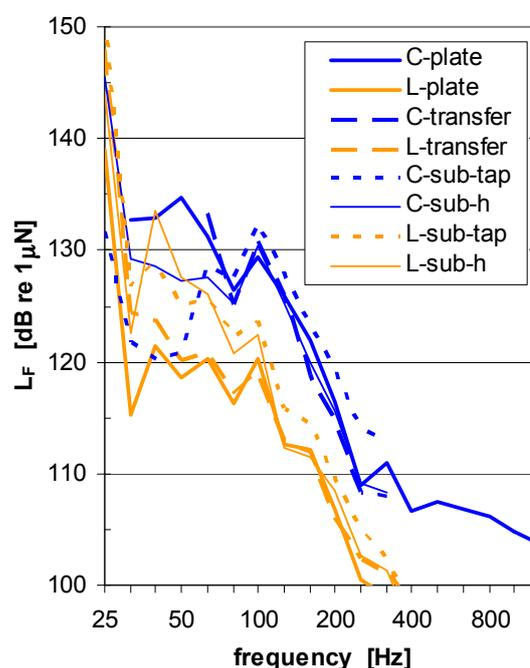
Fig.8 Force level of the washing machine as determined with different methods on the two different floors.
