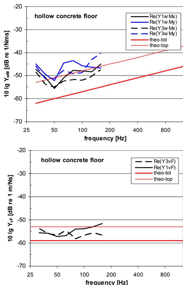
Fig.2 Real part of moment and force mobility of hollow concrete floor.
