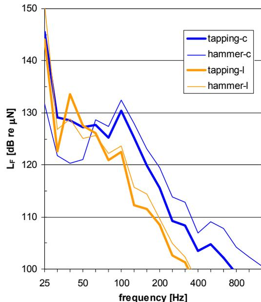
Fig.5 Force level of the washing machine as determined by the substitution method using the tapping machine or calibrated hammer blows on two floor types: concrete and light weight.
