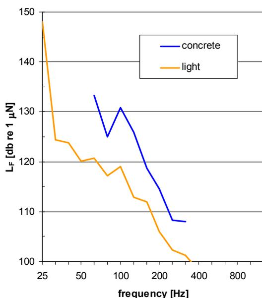
Fig.6 Force level of the washing machine as determined by transfer mobility method on two floor types: concrete and light weight.
