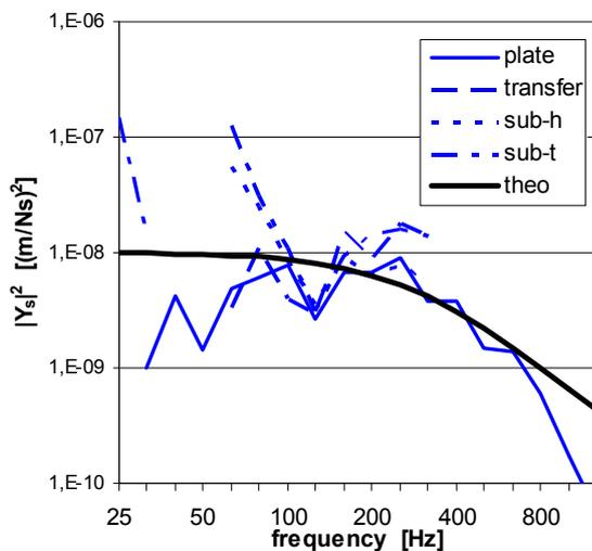
Fig.8 Magnitude of source mobility of the washing machine as determined from different measurement methods on the concrete and the light floor; theoretical value for a damped mass.
