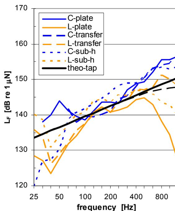
Fig.7 Force level of the tapping machine as determined with different methods on the two different floors; comparison with theoretical value.
