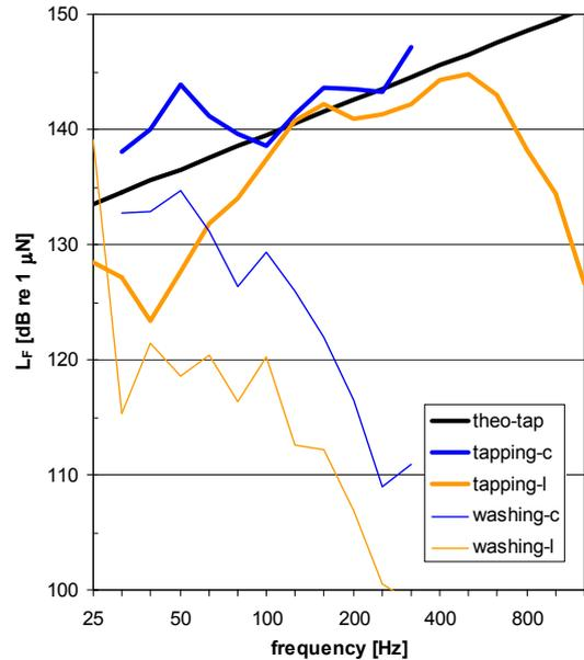
Fig.4 Force level as determined by the reception plate method with tapping machine and washing machine on two floor types: concrete and light weight; theoretical value for tapping machine for comparison.
