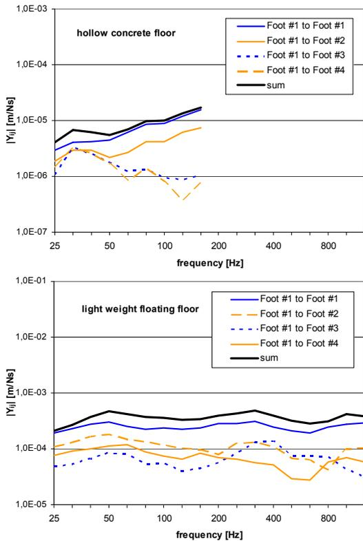
Fig.4 Magnitude of point and transfer mobility between four machine contact points on light weight and concrete floor; square-root of sum as in Eq. 5 also indicated.
