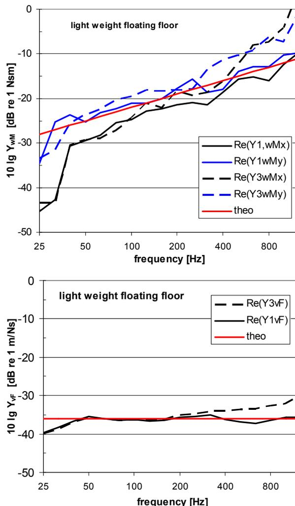
Fig.3 Real part of moment and force mobility of light weight floating floor.
