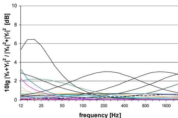
Fig.1 Error in simplification by Eq. (3) for various mobility types for source and receiving structure.
