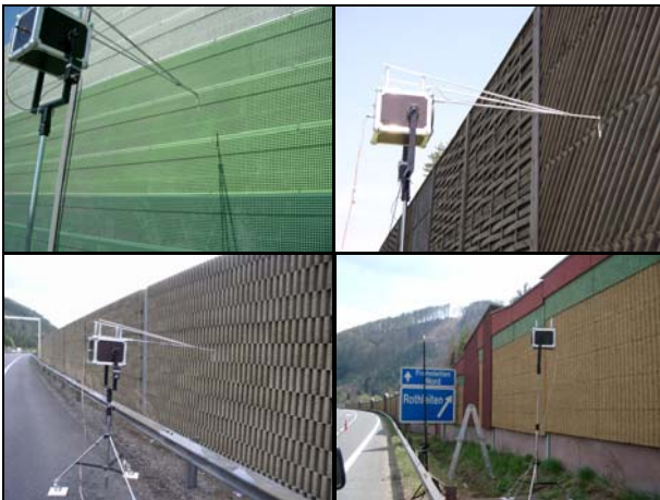
Fig.3 Test equipment during the measurements on the most common Austrian noise barriers (made of aluminium, timber and cement-bound wood chipping).
