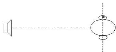
Figure 7: Measurement of the leak. The loudspeaker is placed at 1m in front of the dummy head. On one ear is the headphone, while the other one is left free
