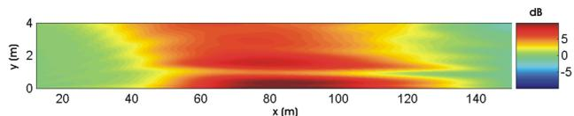
Fig.4 Improvement (dB) in barrier efficiency by the presence of a row of coniferous trees, for the 1000-Hz octave band ( $u^*=0.8$  m/s,  $k_r=2$ ).
