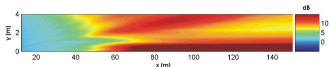
Fig.2 Magnitude (dB) of the screen-induced refraction of sound by wind near a 4-m high noise barrier (at  $x=0$  m), for the 1000 Hz octave band ( $u^*=0.8$  m/s).
