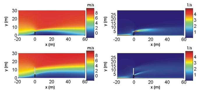
Fig.1 Fields of the horizontal component of the wind speed ( $u_*=0.8$  m/s) (on the left) and fields of the vertical gradient in the horizontal wind speed (on the right), near a 4-m high noise barrier. The figures above depict the situation in absence of trees, the figures below show these fields when a row of coniferous trees is situated directly behind the noise barrier. The canopy extends 8 m above the noise barrier ( $u_*=0.8$  m/s,  $k_r=2$ ).
