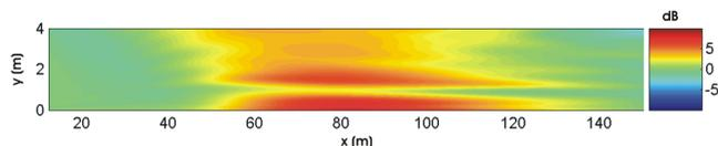
Fig.3 Improvement (dB) in barrier efficiency by the presence of a row of deciduous trees, for the 1000-Hz octave band ( $u^*=0.8$  m/s,  $k_r=2$ ).
