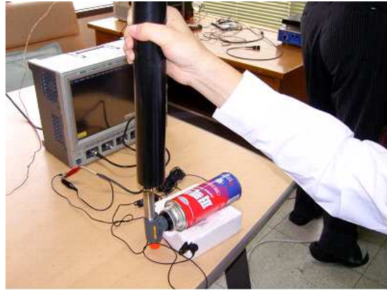
Figure 5: Rijke tube used in the present work. Length of tube was 49 cm.
