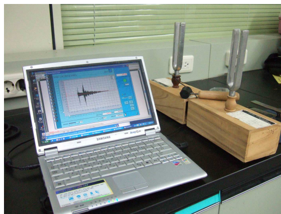
Figure 2: Experimental setup for beat of two tuning forks.
