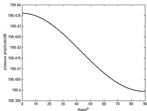
Fig.2. Radiated sound pressure amplitude of the 1/4 circle which is 1m from the center of the transducer in the  $Y=0$  plane.
