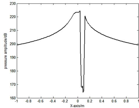
Fig.9. Radiated sound pressure amplitude of the field points on the X-axis.
