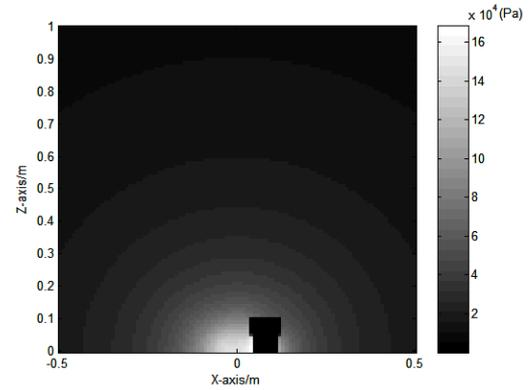
Fig.8. Radiated sound field distribution of the transducer array in the Y=0 plane.
