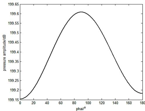
Fig.7. Radiated sound pressure amplitude of the 1/2 circle which is 1m from the origin point in the Y=0 plane.
