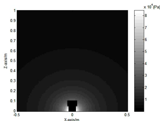
Fig.3. Radiated sound field distribution of the transducer in the  $Y=0$  plane.
