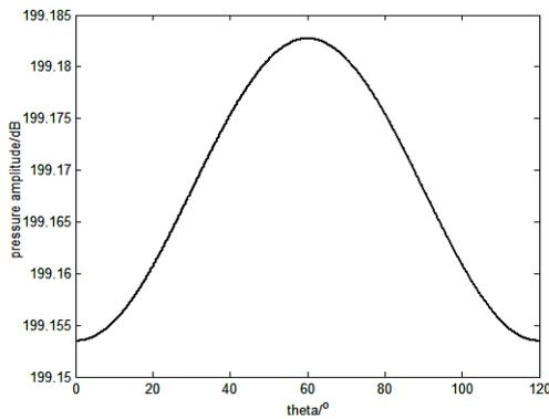
Fig.6. Radiated sound pressure amplitude of the 1/3 circle which is 1m from the origin point in the Z=0 plane.
