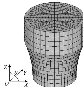
Fig.1. Boundary element model and mesh of upside half-part of the transducer.
