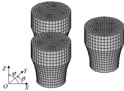
Fig.5. Boundary element model and mesh of upside half-part of the transducer array. (Leftside is the sketch map of coordinate. The origin point is the center of the circle passing the centers of three transducers.)
