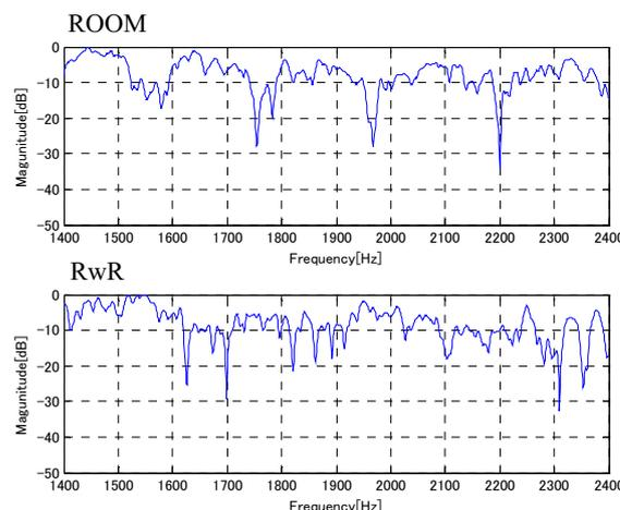
Fig.11 Transfer Function ROOM, RwR ( $S_1-M_1$ )
