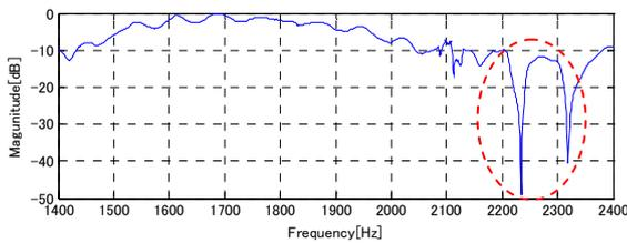
Fig.14 Transfer Function PIPE (S<sub>1</sub>-M<sub>1</sub>)
