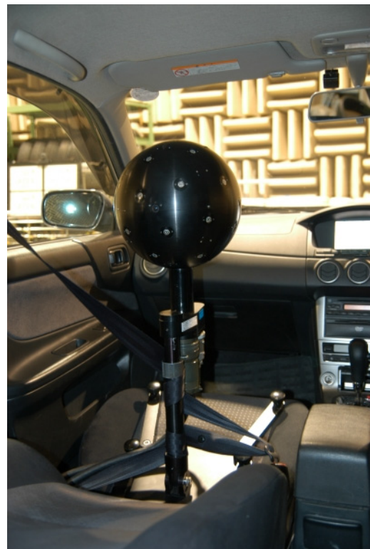
Fig.2 Rigid spherical microphone array in a vehicle
