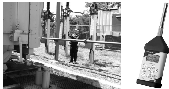
Fig. 1 Measuring appliance (SVAN 945A) used for measurements at the electric power station
