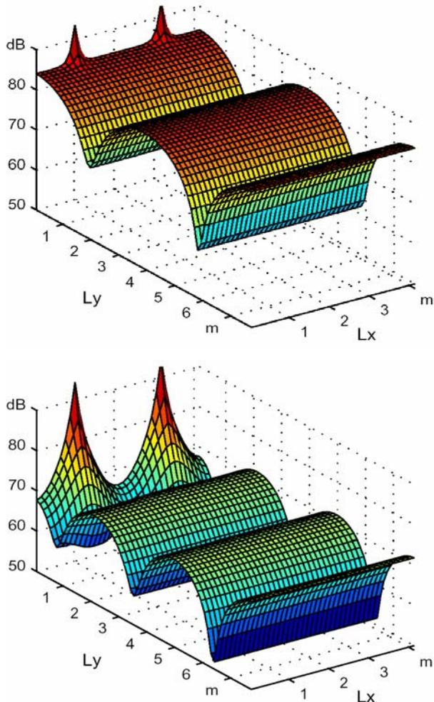
Fig.3: Sound pressure level distribution from a simulation of room A (see Fig. 2) at the height of  $z = 1.38\text{m}$ . Upper at 44 Hz a resonance frequency. Bottom at 60 Hz. The loudspeaker setup is 0.2.0. (see chapter 4.1)
