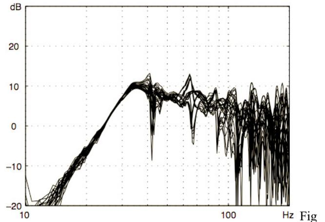
Fig.11: Measurements in room A with CABS 0.2.2 with frequency response at 25 positions.
