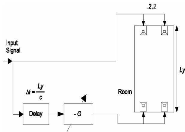
Fig.7: Block diagram of the implementation of CABS 0.2.2 to minimize the reflection from the back wall.
