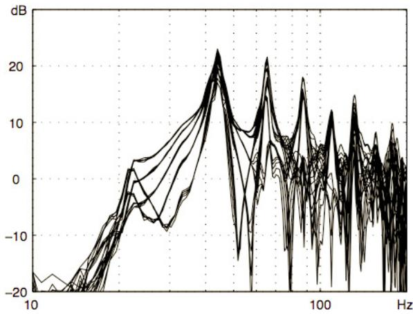
Fig.9: Measurements in the IEC room (room A) with CABS 0.2.0 with frequency response at 25 positions.
