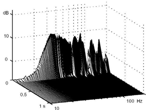
Fig.12: Cumulative spectra decay measured at position 17 with CABS 0.2.2 in room A.
