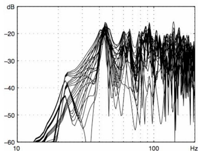
Fig. 1: Simulation of room A with 25 virtual microphone positions and a subwoofer on the floor in a frontal corner
