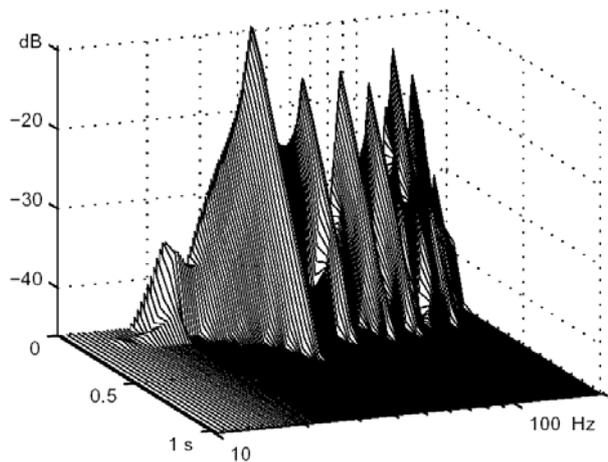
Fig.5: Simulated Cumulative Spectra Decay, room A
