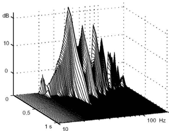
Fig.10: Cumulative spectral decay (CSD) measured at one position (17) with CABS 0.2.0 in the IEC room (room A).
