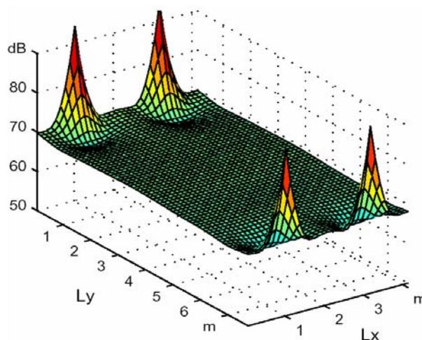
Fig.8: Sound level distribution from a simulation of room A with CABS 0.2.2 at a height  $z = 1,38$  m .
