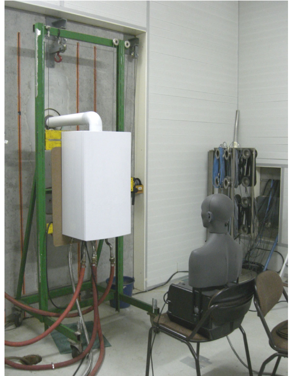
Figure 1: Recording of a wall boiler
