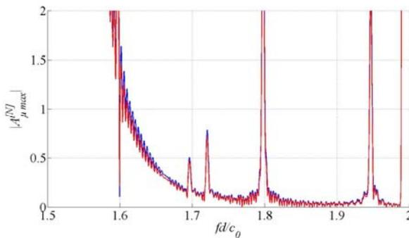
Fig.6 Modulus of the normalized amplitude  $\hat{A}_{\mu=3}^{[5]}(x)/\hat{A}_m^{(0)}$  of the mode  $\mu = 3$  for a sinusoidal profile, as a function of the frequency, without dissipation (upper blue curve) and with dissipation (lower red curve).
