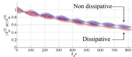
Fig.5 Modulus of the normalized amplitude  $\hat{A}_{m=1}^{[3]}(x)/\hat{A}_m^{(0)}$  of the mode  $m=1$  for a sawtooth profile, as a function of the abscissa of the corrugation, without dissipation (upper blue curve) and with dissipation (lower red curve).
