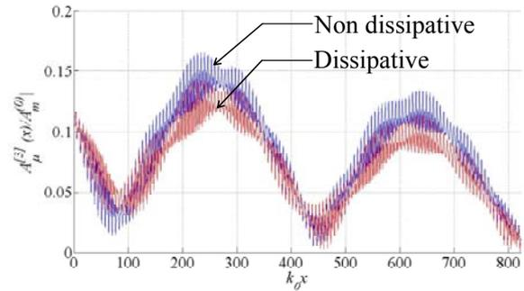
Fig.4 Modulus of the normalized amplitude  $\hat{A}_{\mu=0}^{[3]}(x)/\hat{A}_m^{(0)}$  of the mode  $\mu=0$  for a sawtooth profile, as a function of the abscissa of the corrugation, without dissipation (upper blue curve) and with dissipation (lower red curve).
