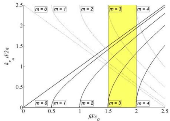
Fig.2 Dispersion curves (solid lines) of the guide with smooth interfaces and curves (dashed lines) corresponding to the phonon relation (21).
