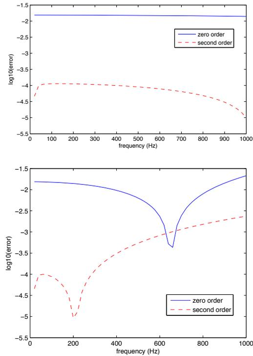
Figure 3: Error versus the frequency for a plane wave at  $10^\circ$  for an element size  $0.01m \times 0.01m$  (upper) and an element size  $0.05m \times 0.05m$  (lower).
