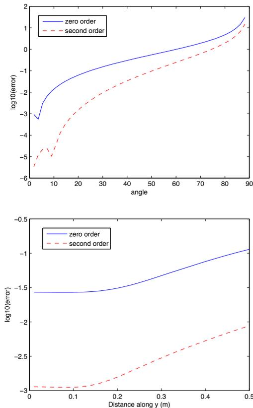
Figure 4: Error versus the angle of incidence (upper) and error versus the distance for a point source (lower).
