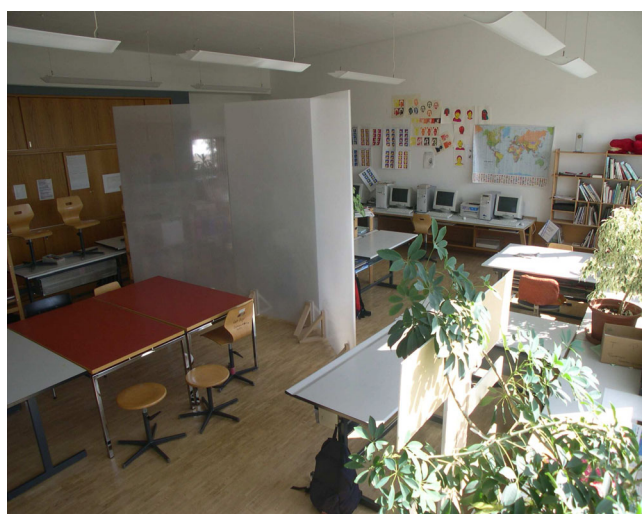
Figure 4: Classroom without (above) and with (below) transparent micro-perforated movable walls.
