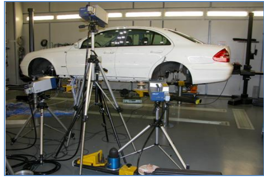
Fig.4 Typical 3D vibrometer setup
