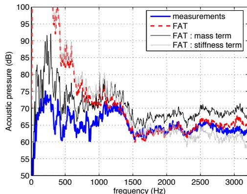
Figure 5: Measured and identified acoustic pressures averaged over the 16 array positions.
