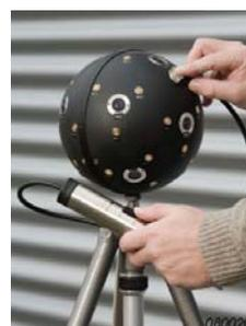
Fig. 5 36 channels spherical array with 12 cameras
