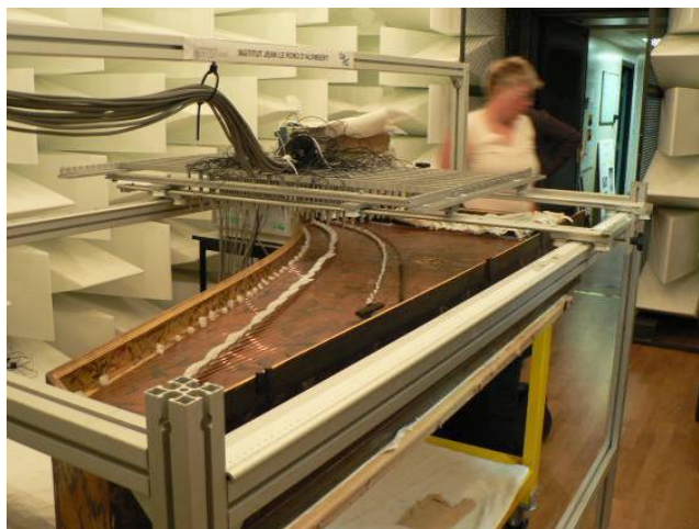
Fig.2. Couchet harpsichord in the anechoic room with string muffling system and holographic microphone array
