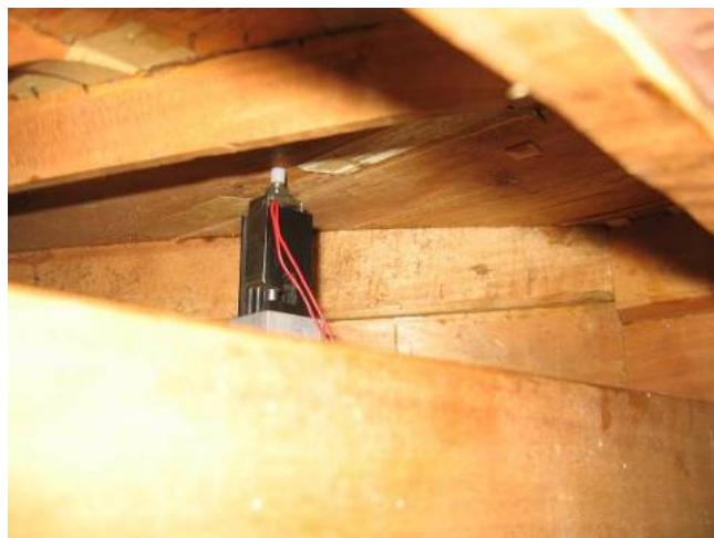
Fig. 4. Impact hammer on position in the harpsichord underside of the soundboard.
