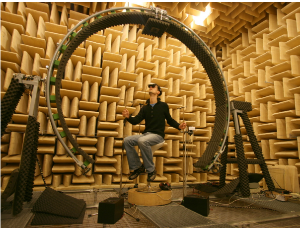
Figure 1: The measurement setup for the sound localisation experiment in the anechoic room. The participant wears a HMD and is seated on a swivel stool. He can turn around 180 degrees to the left and the right. The loudspeaker is attached to a trolley and can move along the hoop that can rotate around the participant. The experiment took place in the dark.
