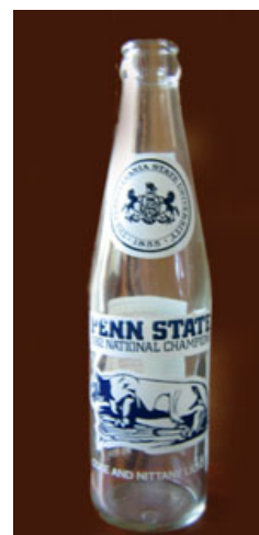
Fig. 6. The neck-length for this bottle is 17.78 mm with a radius of 8.26 mm. The volume is a cylinder that is 12.7 cm long with a radius of 24.38 mm. The length of the conical section that joins the neck to the volume is 10.0 cm.
