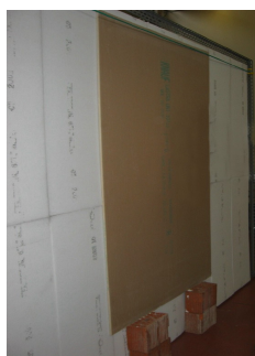
Fig. 13 – Measurement with gypsumboard ref. surface (the picture shows the back of the measurement plane)
