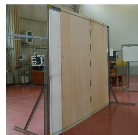
Fig. 10 – Measurement with plywood reference surface (the picture shows the back of the measurement plane)
