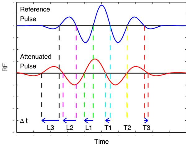
Figure 1. Since the attenuated pulse is low-pass filtered (stretched in time) due to frequency-dependent attenuation of the bone,  $\Delta t$  varies with marker location. Transit-time markers are labeled L3, L2, L1, T1, T2, and T3 where L and T denote the leading and trailing halves of the pulse and markers are numbered outward from pulse center.
