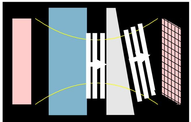
Figure 4. From left to right: 1) transmitter, 2) bone-mimicking phantom, 3) acrylic wedge, 4) receiver. The wedge deflects wavefronts, resulting in phase cancellation.
