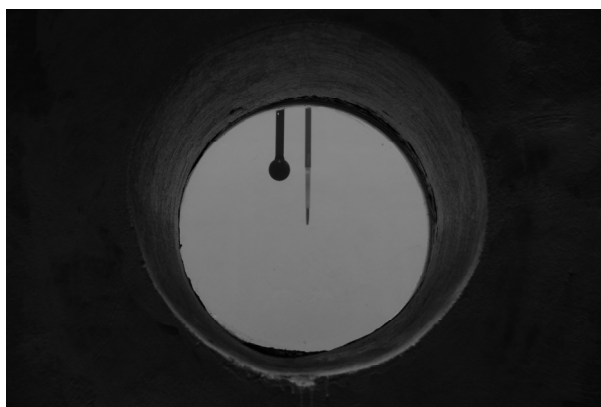
Fig. 2. Two windows are provided on one of the tank walls for combined optical and acoustical measurements (in addition to the accredited ones), which can be performed using the available 16-mm film rotating prism high-speed camera (up to 10 000 frames per second) and the Laser Doppler Vibrometer (up to 100 kHz), respectively.
