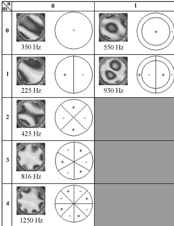
Fig. 2 Velocity maps of the modes in the pressure plate of the VS 1.6 (reproduced from Ref. 4).
