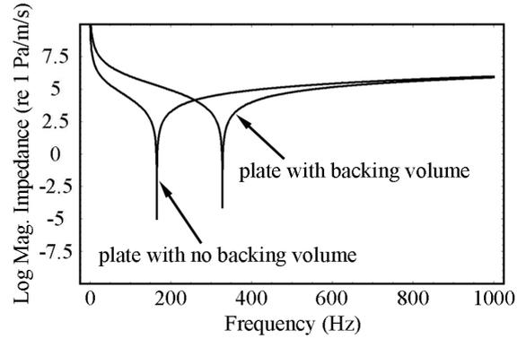
Fig. 7 Plot of the impedance of the (0,0) mode of an elastically supported plate with and without a backing volume (reproduced from Ref. 4).
