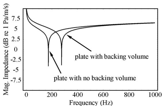
Fig. 8 Plot of the impedance for the (0,1) mode of a clamped plate with and without a backing volume (reproduced from Ref. 4).
