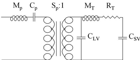
Fig. 6 Electrical equivalent circuit for the (0,0) mode of the VS 1.6 (reproduced from Ref. 4).
