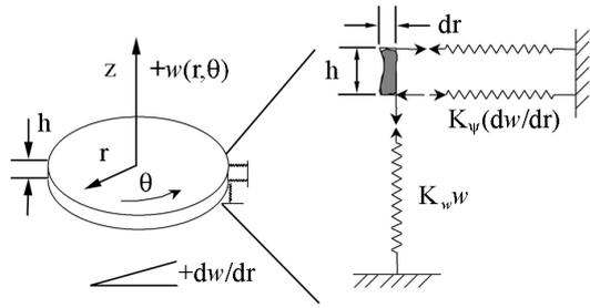
Fig. 5 Geometry of the elastically supported plate model (reproduced from Ref. 4).
