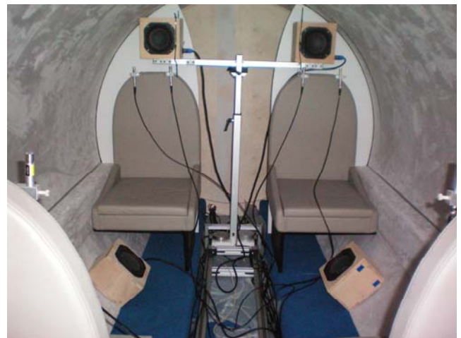
Fig. 9 Acoustic mock-up interior with the experimental ANC system (view towards cabin rear from 1. seat row).
