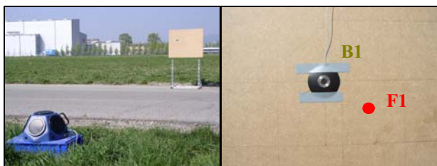
Fig.1 Left the setup of the measurements with the BB (backing board), right the surface microphone during the measurement at position B1 (in red also position F1).
