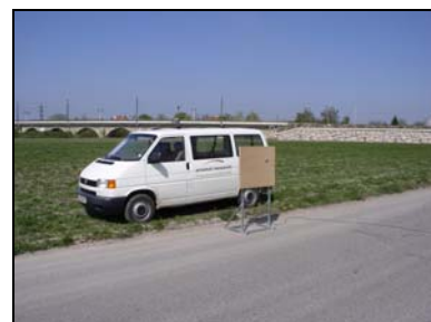
Fig.7 Experimental setup for the measurements with a reflecting object near to the backing board.
