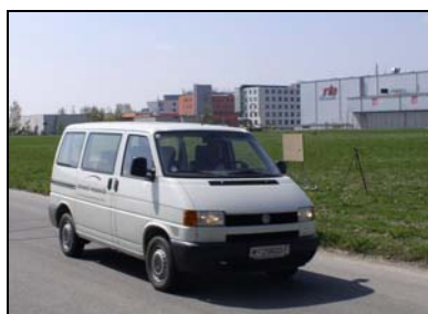
Fig.9 Setup for the pass-by measurements at 60 km/h (simultaneous measurements with the surface microphone on the board and with the free-field microphone for the pass-by measurement).
