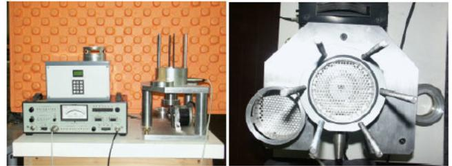
Fig.3 (a, b) Apparatus for the measurement of the airflow resistance in porous and fibrous materials according to Standard EN 29053, made at INRIM of Turin.
