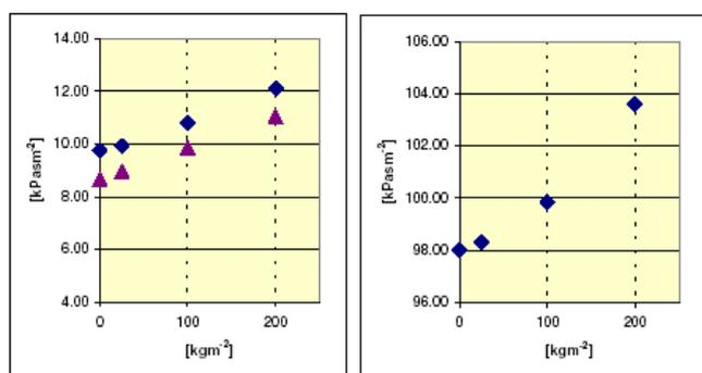
Fig.6 (a, b) The airflow resistivity as a function of applied load.
