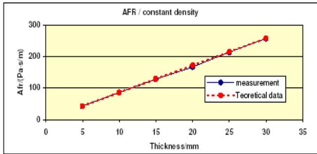
Fig.1 Experimental verification of linear variation of the resistance to flow depending on thickness at constant density.
