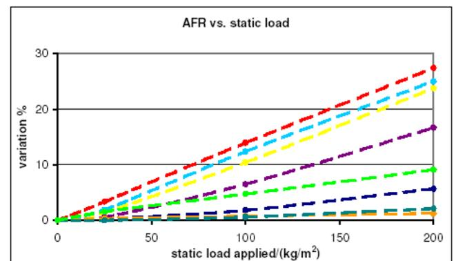
Fig.5 Percentage variation of airflow resistivity, as a function of the applied load, in various typologies of materials used as insulation in floating floors.
