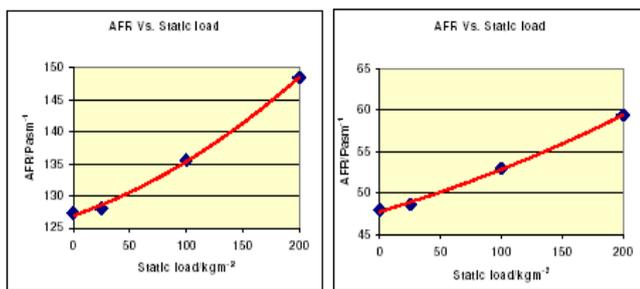
Fig.2 (a, b) Experimental verification of the airflow resistance variation depending on the thickness decrease (or density increase) in two materials subject to a compression under static load.
