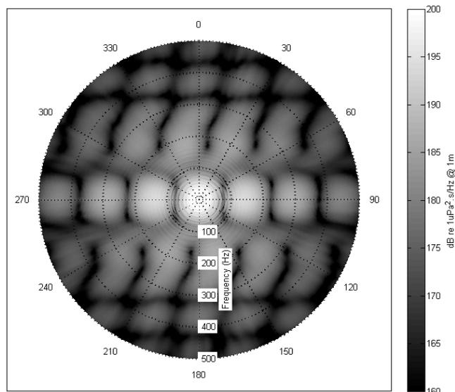
Fig. 3. Modelled horizontal plane beam pattern for a commercial airgun array. Frequency increases radially from the centre. Gray-scale represents source spectral level. An azimuth of  $0^\circ$  corresponds to the tow direction. Surface reflection is not included.
