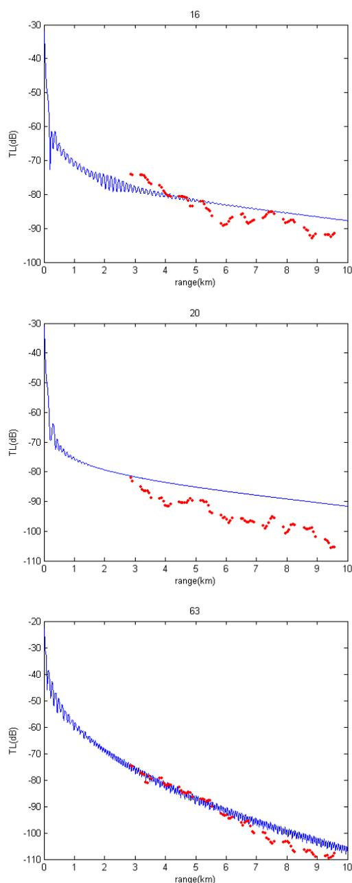
Fig. 7 Measured (points) and modelled (line) transmission loss vs. range for optimised parameters from run 1 for frequencies of 16 Hz (top), 20 Hz (middle) and 63 Hz (bottom).
