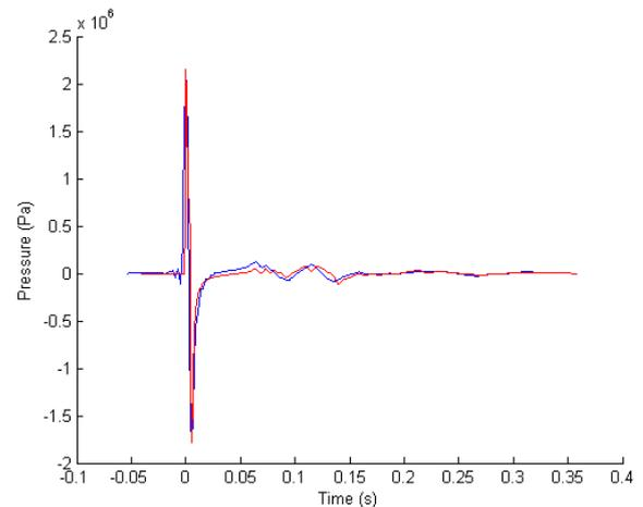
Fig. 2 Comparison of two different simulations of the signal produced by a commercial airgun array with a total volume of 28.8 litres. Plot is for the vertically downward direction and includes the effect of the surface reflection.
