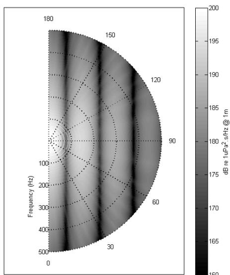
Fig. 4. Modelled vertical plane beam pattern for the same array as Fig. 3 in the array broadside direction ( $90^\circ$  azimuth). An elevation of  $0^\circ$  is vertically downward. Surface reflection is not included.
