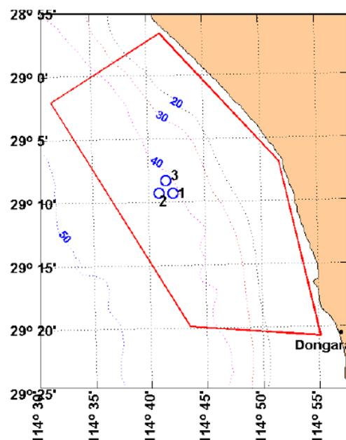
Fig. 5 Case study seismic survey location. Solid lines indicate boundary of seismic survey, dotted lines are depth contours with depths given in metres. Circles show locations of autonomous recording systems. Data from recording system 1 were used for this study.
