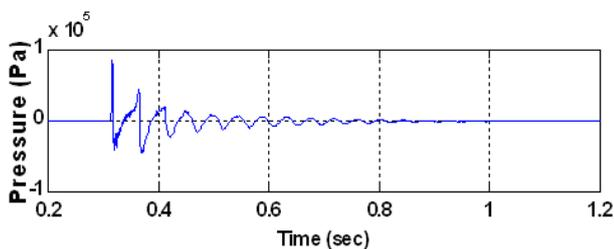
Fig. 1 Acoustic signal recorded 0.87m from a 0.33 litre (20 cui) airgun operating at 10 MPa.
