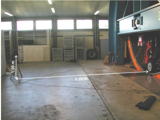
Figure 5: experimental set-up of indoor drum test facility and microphone position
