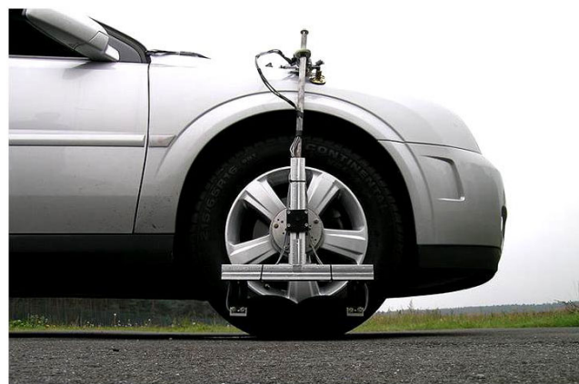
Figure 9: Side view of sound intensity probes mounted on a vehicle
