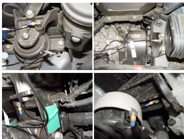
Fig.3 Setup of accelerometers at each mount bracket
