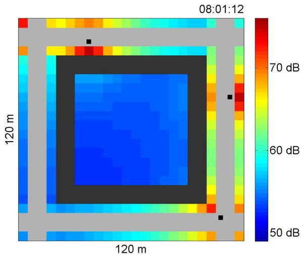
Fig. 9. Snapshot of the sound field at time 8:01:12. The region is located at the center of the city.
