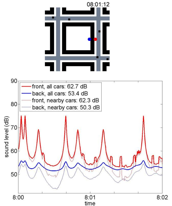
Fig. 10. Sound level as a function of time from 8:00 to 8:02, for two receivers: a receiver at the front of the buildings along a street (red dot in the snapshot above the graph) and a receiver at the back (blue dot in the snapshot). Also included is the contribution from cars within 200 m distance from the receiver. Average levels over the period of two minutes are indicated in the legend.
