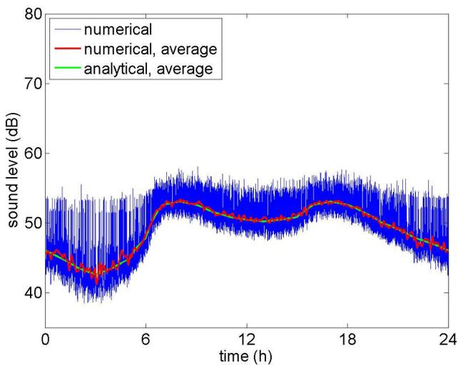
Fig. 11. Sound level as a function of time for a complete period of 24 h, for the receiver at the back of the buildings (see Fig. 10). The blue line represents the direct result of the numerical simulation. The red line represents a running average over intervals of 6 minutes. The green line represents the analytical solution for the average sound level as a function of time.
