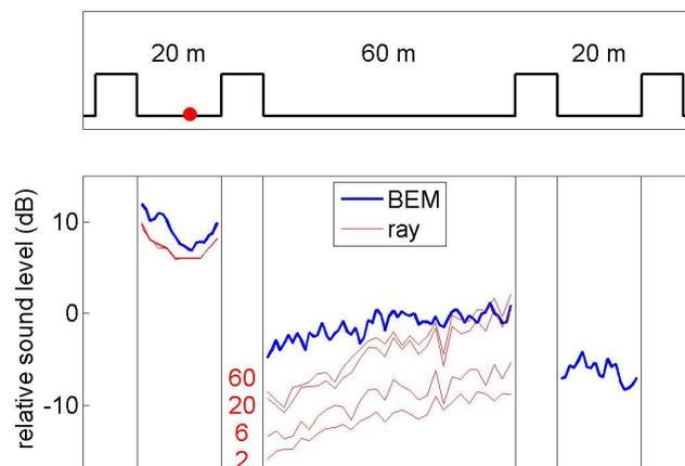
Fig. 6. Relative sound level as a function of position along a cross section of the model city shown in Fig. 4, calculated with a BEM model and a ray model with 2, 6, 20, and 60 canyon reflections. Heights of source (red dot) and receiver are 0.5 m and 0 m, respectively. The sound level is averaged over frequency range 80-730 Hz, using relative traffic noise emission levels of -8.4, -5.4, and -2.4 dB for octave bands 125, 250, and 500 Hz, respectively.
