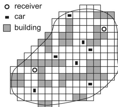
Fig. 2. Representation of a city by a grid of square cells.
