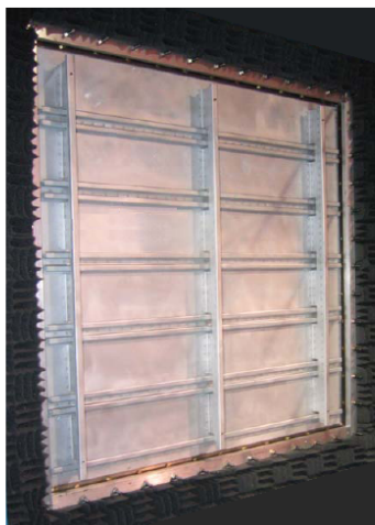
Figure 3: Photograph of the stiffened aluminum test panel.
