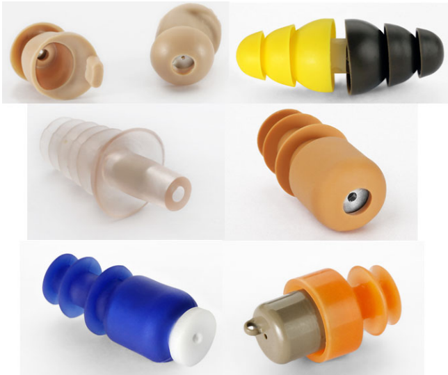
Figure 3 – Earplugs tested in this study as described in Table 1. Gunfender (back and front view), Combat Arms, Noise Braker, Ear Valvs, Sound Baffler, and Quiet Please (left to right, top to bottom).
