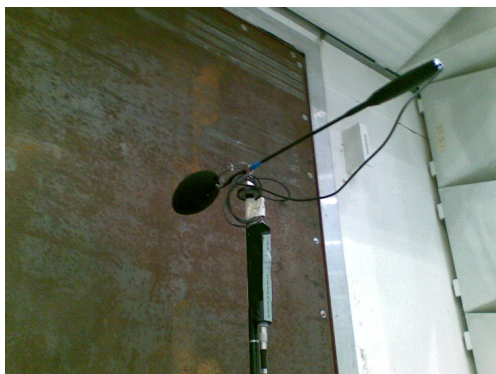
Figure 3: Intensity probe used for the ISO 15186 tests
