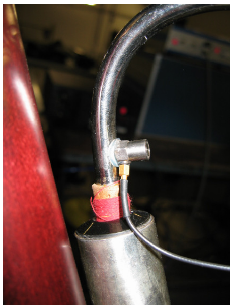
Figure 3: Accelerometer attached to the S-tube.
