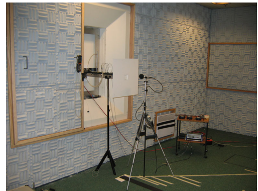
Fig. 8 : Duct termination with automotive outlet connected to the blower but placed in an acoustically treated room
