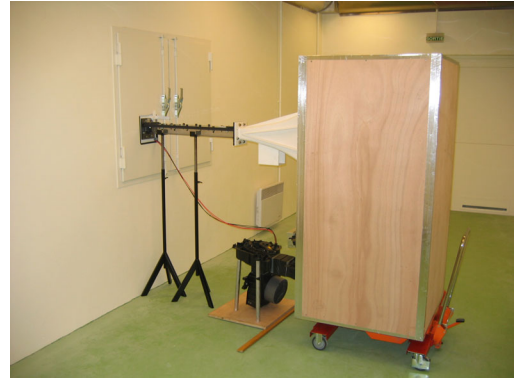
Fig. 7 : Blower and expansion chamber generating the quiet flow isolated in a separated room
