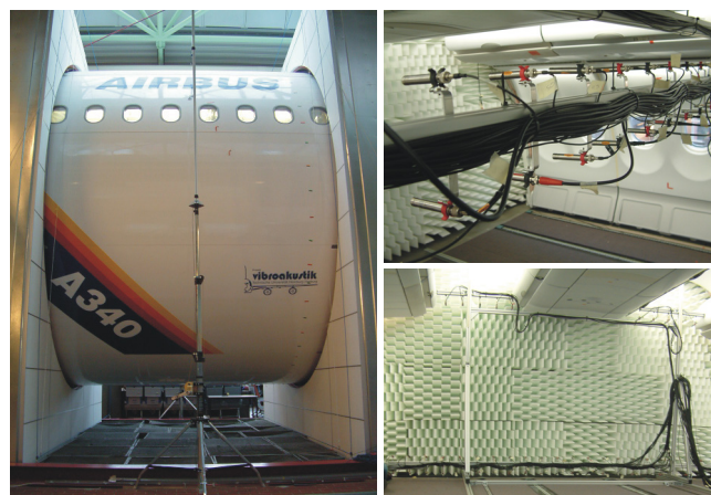
Fig. 6: Aircraft mock-up (left), measuring apparatus (right)
