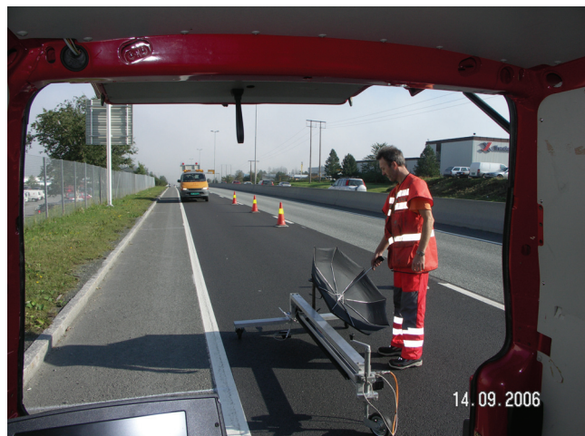
Fig.1 3D Texture measurement rig
