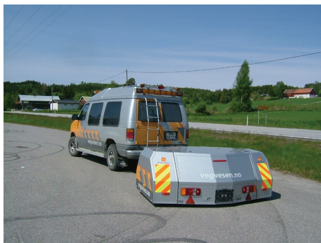
Fig.2 CPX-trailer used for measurements
