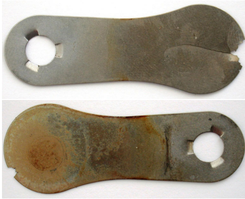
Figure 7: Damage (Cracks) of the two 0,2 mm thin reeds
