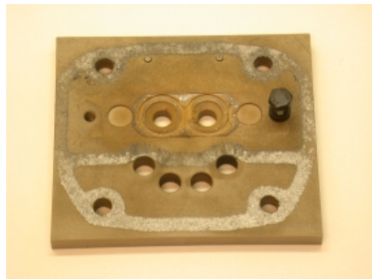
Figure 2: Valve plate made of G lass fibre R einforced P lastic (GRP)
