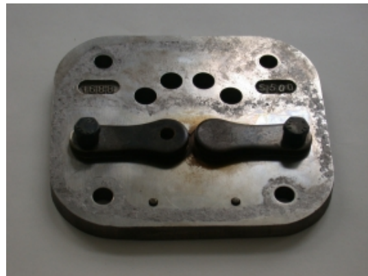
Figure 1: Conventional valve plate made of steel
