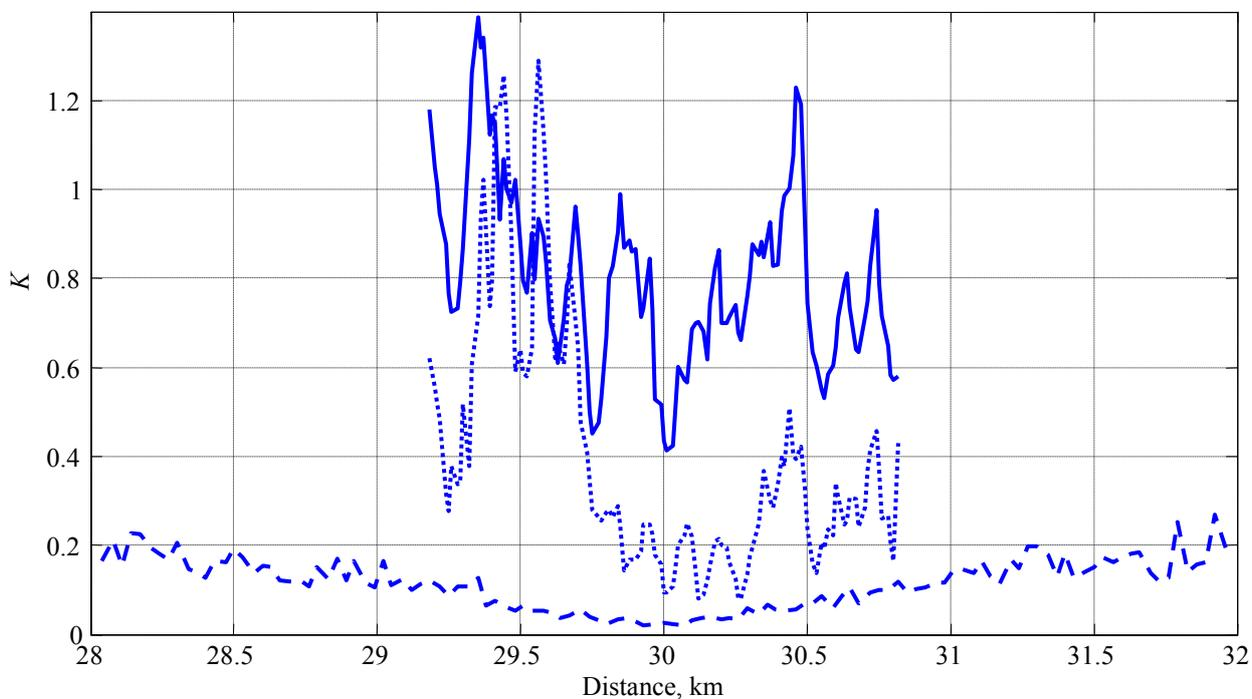
Fig.5. Ratio of magnitudes of scattered signals for focusing to the waveguide center and sea bottom. The dashed curve corresponds to wintertime hydrology, dotted and solid curves correspond to summertime hydrology without and with internal waves, respectively.
