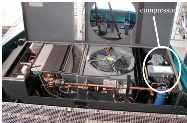
Fig. 1: General view of the HVAC unit mounted on top of a tram roof.
