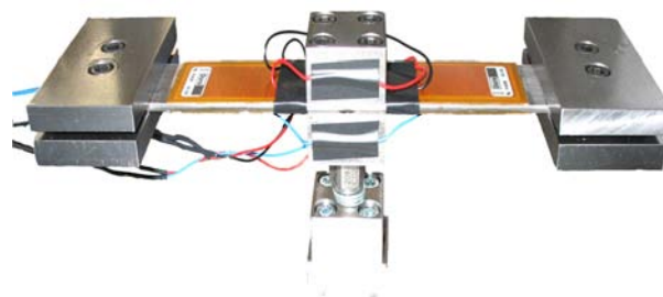
Fig. 14: Prototype of an active tuned vibration absorber.
