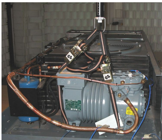
Fig. 3: Compressor suspended from a flexible rope.
