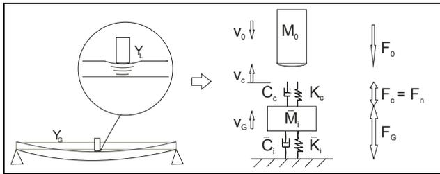
Fig. 2: Description of the excitation by the local and global parts of the admittance  $Y$  at the driving point
