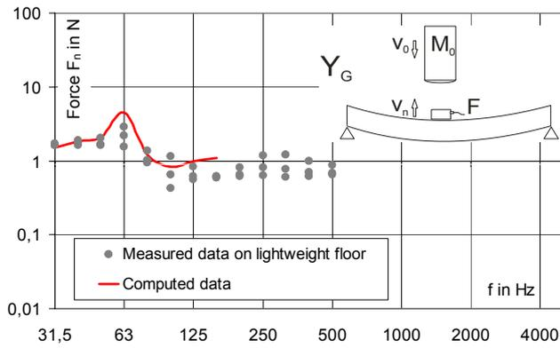
Fig. 4: Excitation force of the tapping machine (single hammer,  $f = 2$  Hz) considering global effects of a lightweight floor for the first eigenmode of the planking at  $f_0 = 80$  Hz (measured 63 – 100 Hz).
