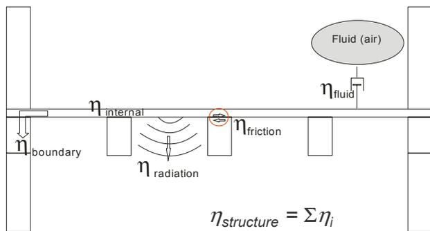
Fig. 5: Different parts of the loss factor
