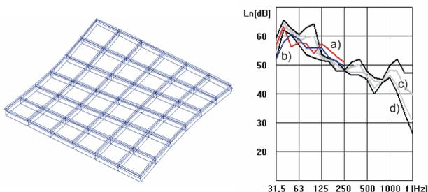
Fig. 12: Comparison measurement – computation for a laminated timber floor with a floating floor screed on mineral wool and crushed stones as loading.
