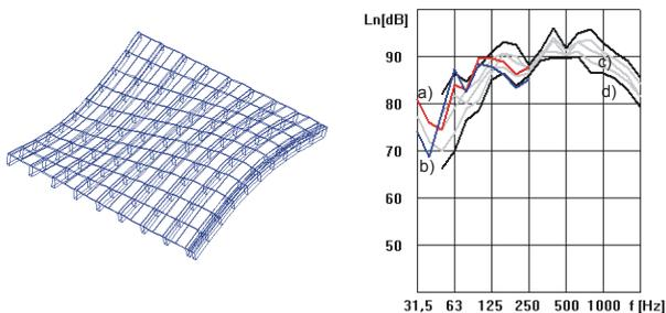
Fig. 11: Comparison measurement – computation for a simple lightweight floor. a) computation using an integral method for the radiation b) computation using a modal method for the radiation c) measured data of similar floors in different test facilities d) mean value of measured data  $\pm 2\sigma$
