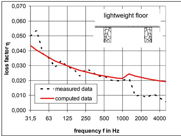
Fig. 7: Comparison between measured and computed loss factor
