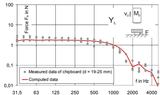
Fig. 3: Excitation force of the tapping machine (single hammer,  $f = 2$  Hz) considering local effects at chipboards with a thickness of 19-25 mm on a stiff base.
