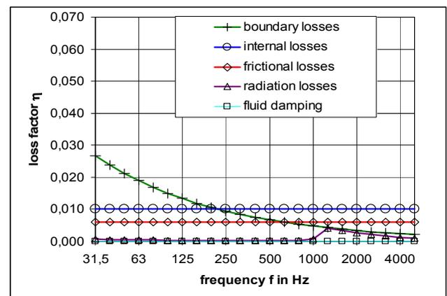
Fig. 6: Computed contributions to the structural damping
