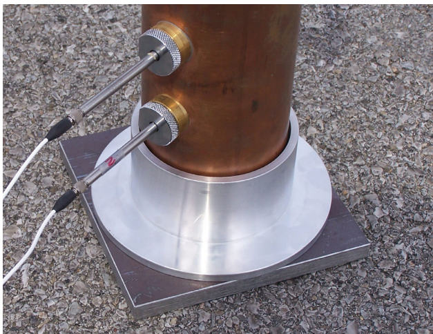
Figure 5: Measurement of tube parasitic absorption.
