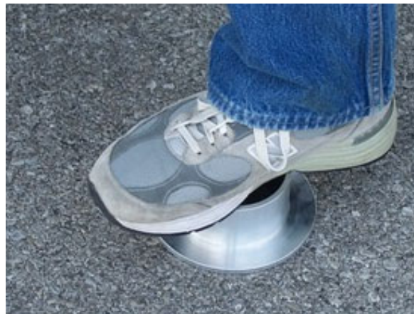
Figure 3: Exerting a uniform 150 kPa on the test fixture at a typical measurement position.
