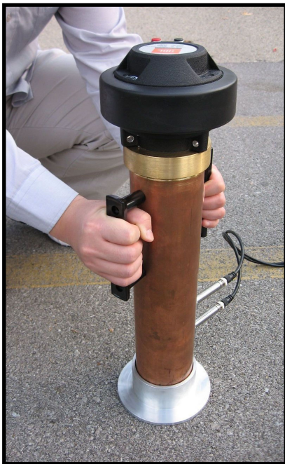
Figure 1: System for measurement of pavement absorption.
