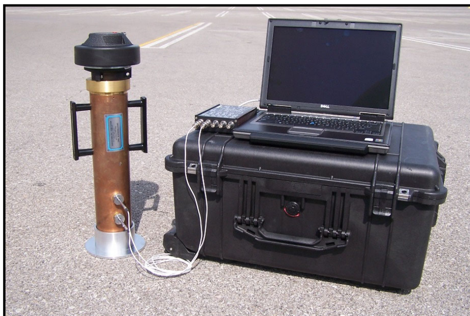
Figure 7: Stand alone system for pavement absorption measurement.
