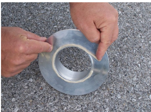
Figure 2: Test fixture showing groove and sealant.
