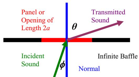
Fig.1 Sound incident at an angle of  $\phi$  to the normal to a panel or opening and radiated at an angle of  $\theta$  to the normal.
