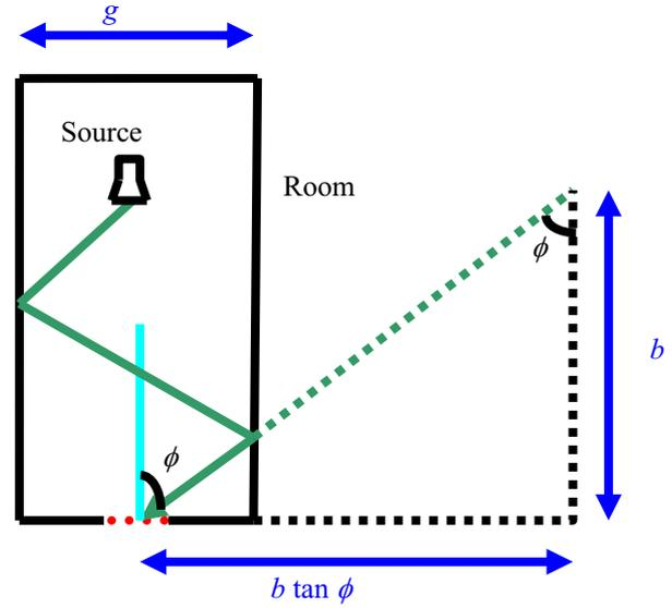
Fig.2 Calculating the number of wall reflections before sound hits the panel or opening at an angle of  $\phi$  to the normal.
