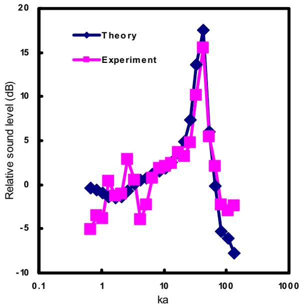
Fig.4 Comparison of the experimental and the theoretical sound pressure level relative to  $0^\circ$  of a 6 mm glass window at  $60^\circ$  as a function of  $ka$ .
