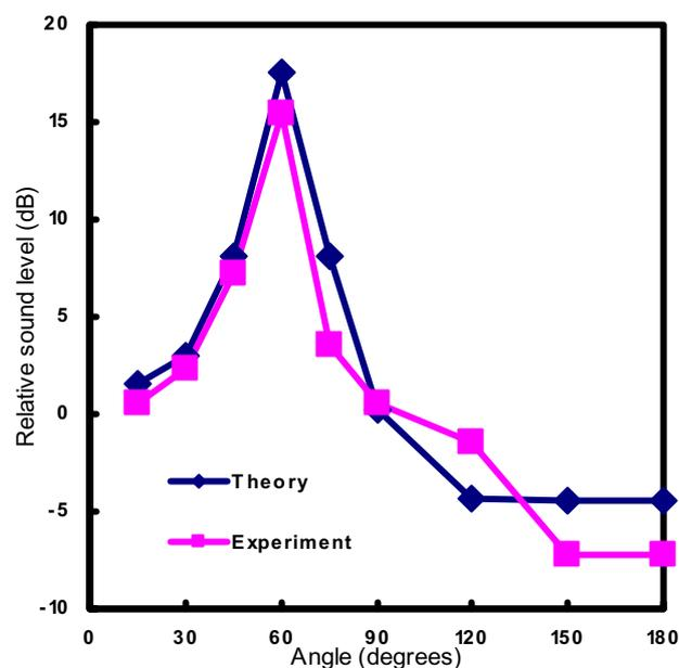
Fig.3 Comparison of the experimental and the theoretical sound pressure level relative to  $0^\circ$  of a 6 mm glass window at 3.15 kHz as a function of angle of incidence.
