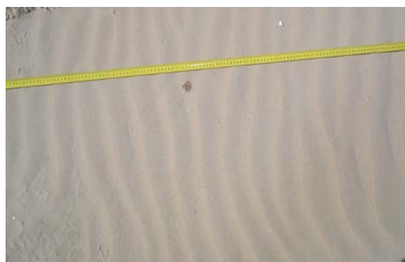
Fig.2 Active ripples forming, \lambda=7-8\text{ cm} , near surface wind velocity=2m/s
