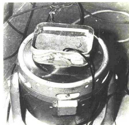
Fig.3.Laboratory experiments had been carried out on vibro table for research VEDS-10A Under research is beach sand, Roja all that process is well traced: the sand activation on horizontal surface, gathering of all sand grains on a surface at an angle, the growth of the angle to maximal and alignment of the surface that corresponds to the amplitude of vibratory acceleration
