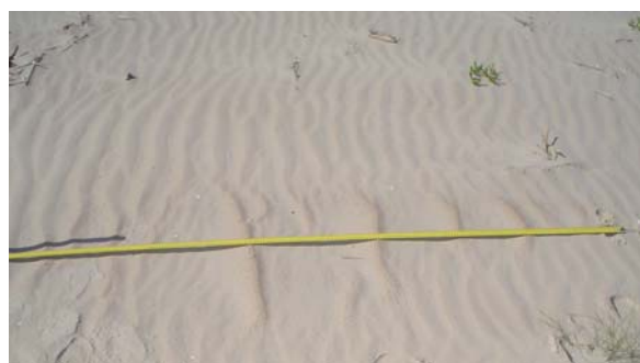
Fig.3 Active ripples forming, \lambda=28-32\text{ cm} , near surface wind velocity = 8 m/s,
